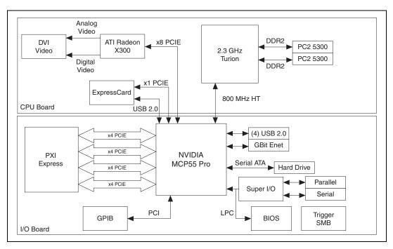
Figure 1-2 illustrates the architecture of the CPU board and the I/O board.
